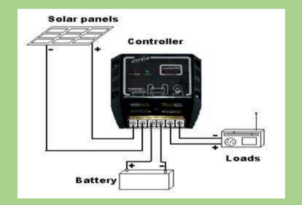
A solar charge controller is available in two different technologies:
